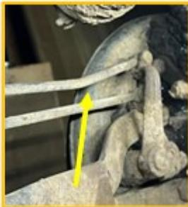
3. Bent brake rod. One in the front also bent.
