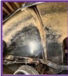
1. Front fender underside. Not bad for 93. Sheet metal intact. No signs of cracking or rot.
