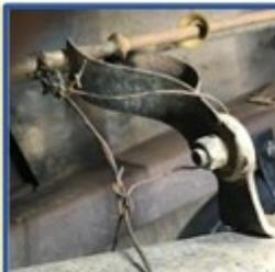
3. I could not find this brake spring baling wire mod in the service bulletins!
