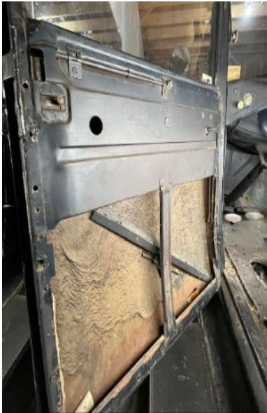
Driver door with trim panel removed. Sagging inner coating
