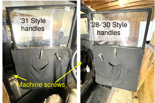
Driver (l) and Passenger (r) side doors. The covering is replacement and the hardware is mismatched. What lurks beneath?
