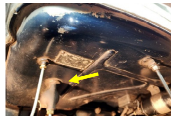
The "indented firewall" refers to a teardrop shape located at the fuel sediment bowl to accommodate move of the fuel cut-off.
