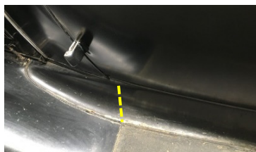
Left side running board/ splash apron. '30 cars have a seam at the yellow line, '31 cars do not.
