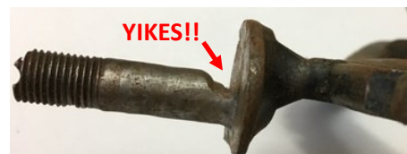
Front motor mount excessive wear. Where do similar problems lurk?
