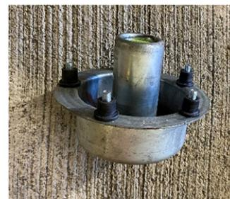
Now all you have to do is press the leveling hub on the wheel (picture below to the left) that needs balancing and then place the wheel on the pedestal (see below right). Balance the tire and install it on the car.
