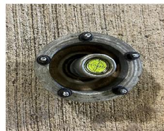
Once that was accomplished, I took the leveling hub to a drill press and drilled a 1/16-inch hole in the center of each of the wheel lug nut holes. At that point I was able to install the rubber spacers onto the leveling hub using 1/16-inch hex bolts. As seen here.
