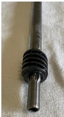
It will be shipped in a tube placed inside a box and padded with crumpled "Kraft" paper. The box is 54" x 5 3/4" x 6 1/2" and weighs 8 lbs., 2.2 oz. The shaft is original from a May 1929 Model A. The worm is likely worn in the middle grooves and should be pressed off and a new worm pressed on (use a new sector gear also). End threads are good. Neither end is damaged. Price \$50 plus shipping from zip code 22124. Please contact: Bud Pratsch at 703-620-2518
