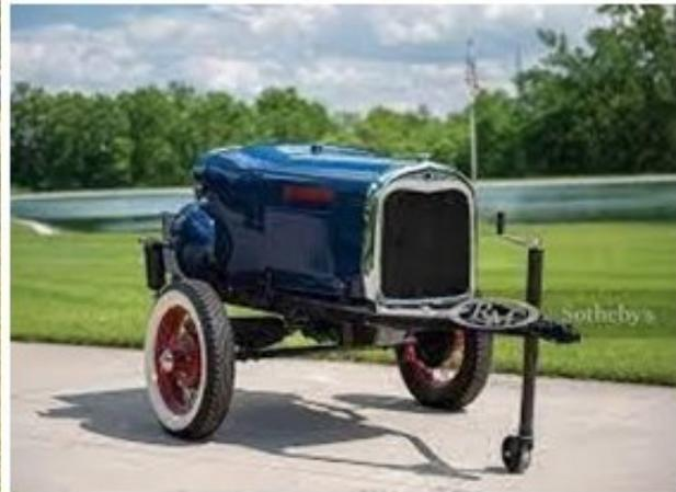
**Manufacturer: Engine Horse Power: Max. Air Pressure: Compressor Type: Gordon Smith Company 20 HP. - 90 PSI. - Single Stage - 6 Volt w/positive Ground Fuel Capacity: 11 Gallons Output: 60 CFM. - Air Tank Size: 65 Gals.**
