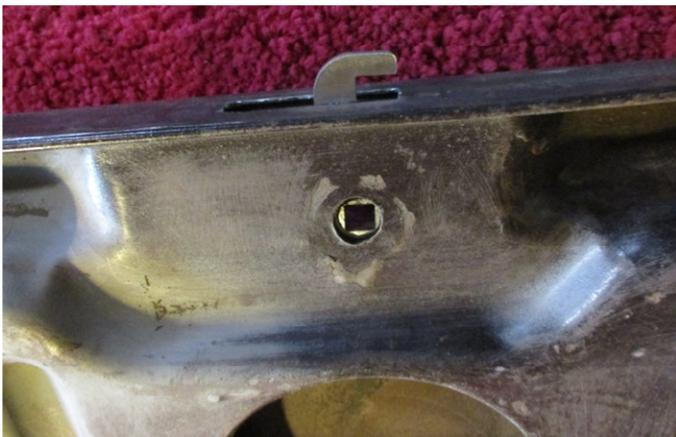
The photo shows the underside of the top of a 28-29 rumble seat lid. You can see the latching arm sticking out of the top of the 28-29 lid. This latching arm swings out to this locking position when the handle is turned. Over time the Ford engineers realized that there was a problem. If the lid is closed while the handle is turned to this closed position, the latching arm strikes the painted surface of the panel ahead of the rumble seat opening.
