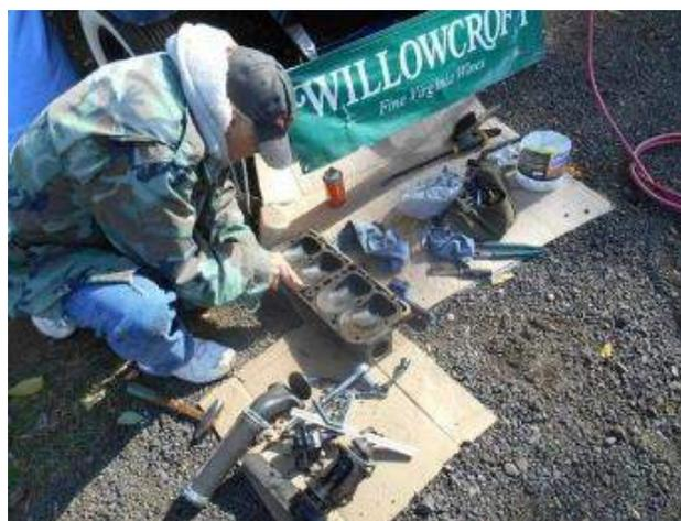
I finish stuffing the holes with rags, while Benny works on the head to scrape off the old gasket.
