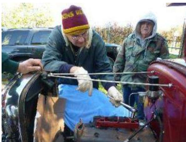
I pull the hose off the goose neck; later, Clem tightens down the nuts on the head puller.
