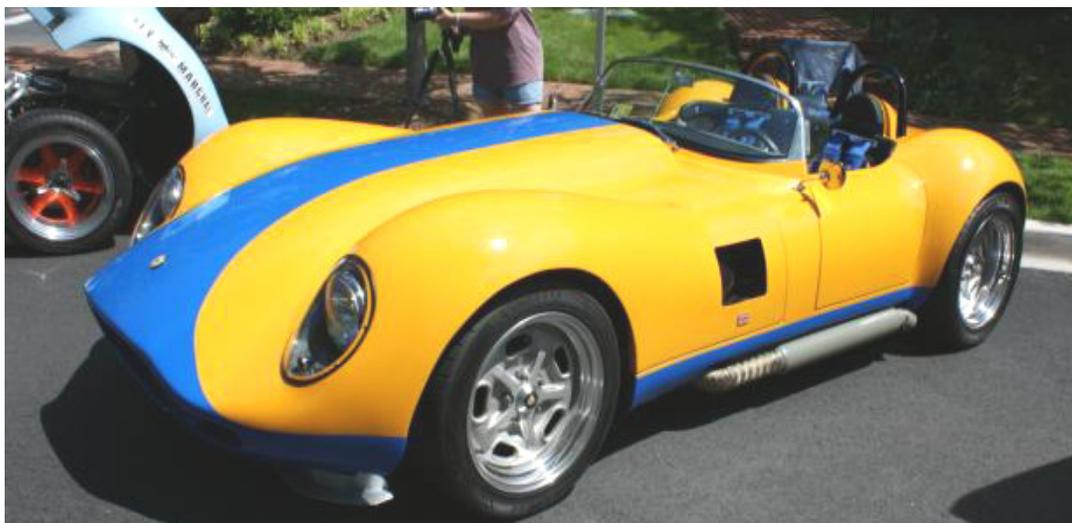
**Custom built body on a '58 Jaguar frame with a 675 hp engine**
