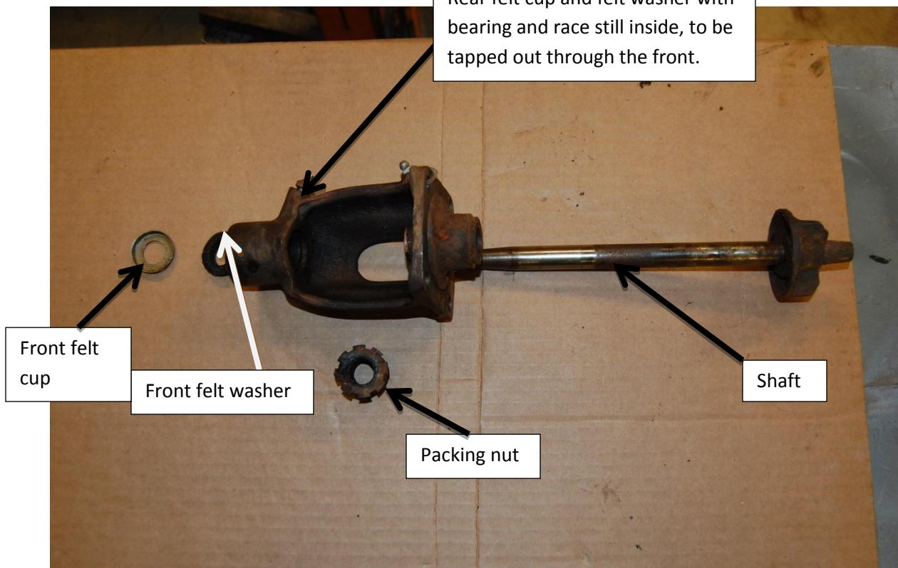
2. Remove felt retainer cup and felt washer from the front, it can be pried out or pulled out. Be careful, as some of old the parts may be need or reused for the rebuild, as modern or reproduction parts often do not fit as well.
