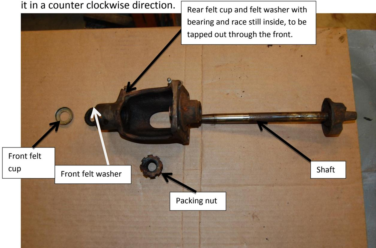
2. Remove felt retainer cup and felt washer from the front, it can be pried out or pulled out. Be careful, as some of old the parts may be need or reused for the rebuild, as modern or reproduction parts often do not fit as well.
