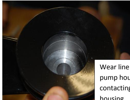
Wear line from pump housing contacting fan housing
