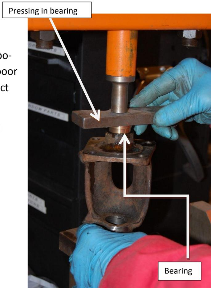
3. Insert the front race and check it with a flash light to verify alignment with the hole in the housing with the hole in bearing race. next grease the fittings to see that the grease is going through the hole in the race, this will assure you that the race is aligned with the housing.
