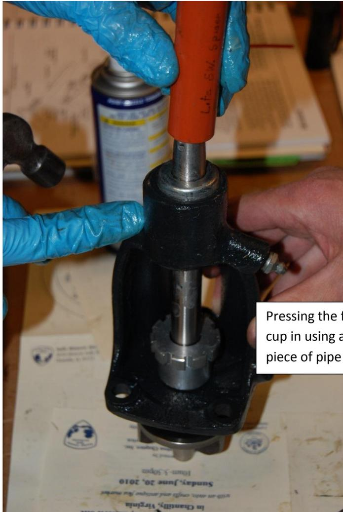
Pressing the felt cup in using a short piece of pipe
